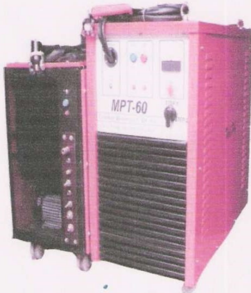
Water cooling unit
